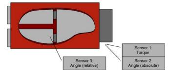
Fig. 10a – Actuator internals – Layout: Schematic drawing explaining internal layout of the actuator, representing interconnections among the components (motors, elastic transmission, output shaft).
